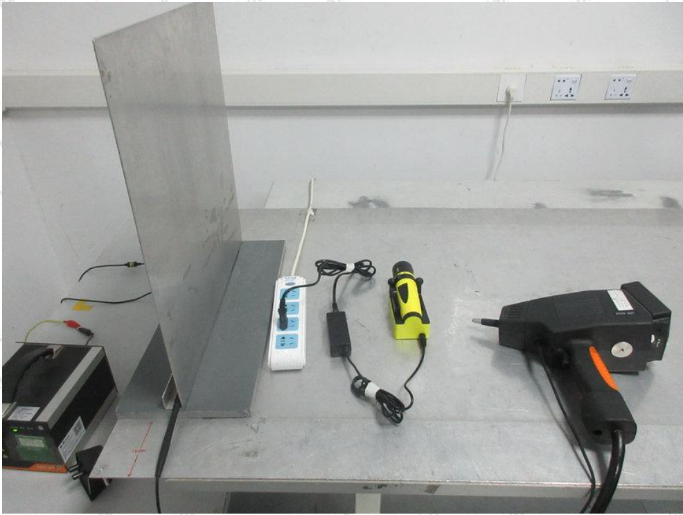
Photo of Electrostatic Discharge Immunity Test (Test Mode: Charging)
