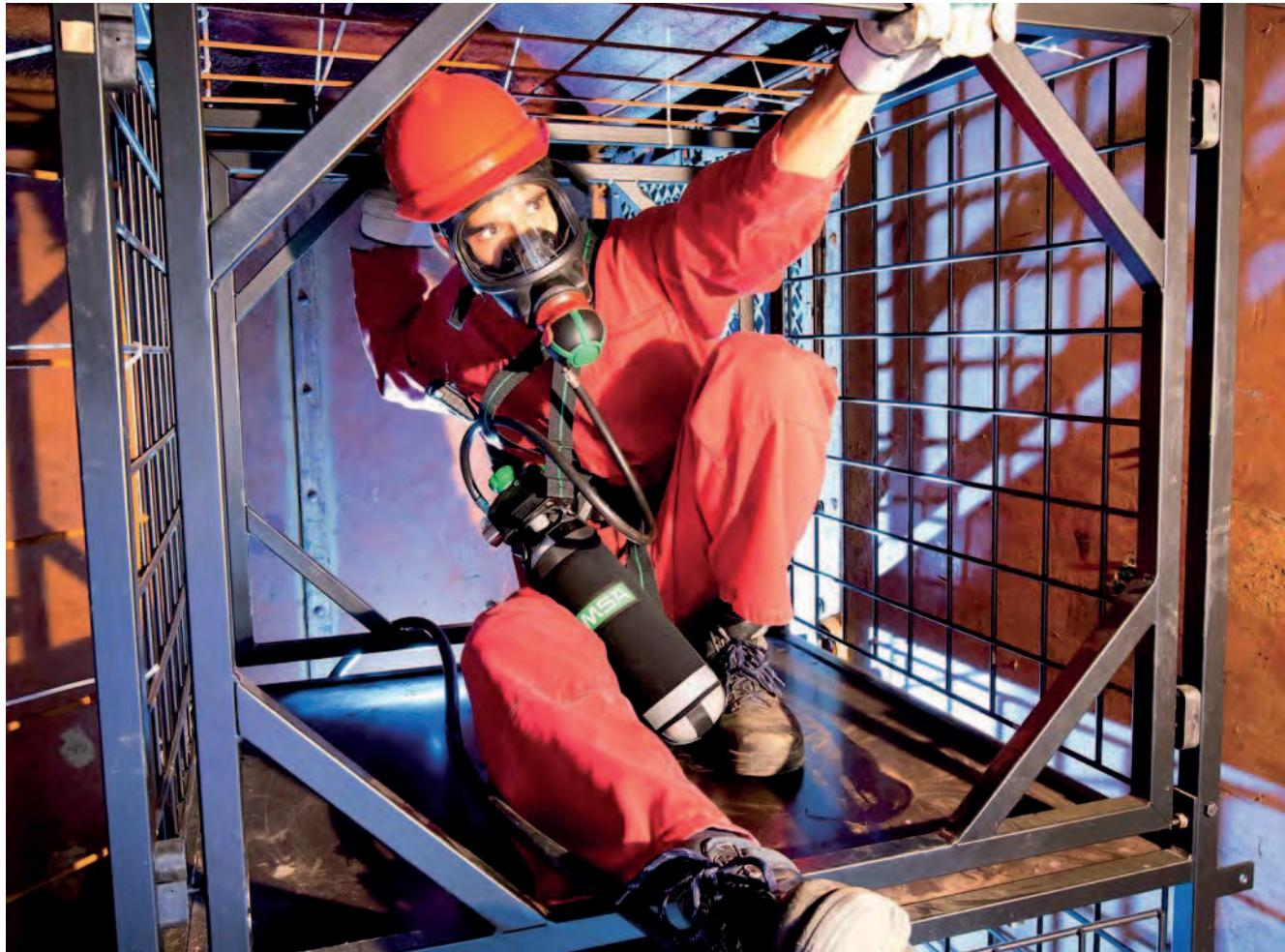
Airline systems are suited for long-duration work restricted to one location or adverse conditions when a confined entry does not permit use of a compressed air breathing apparatus. You can choose between compressed air systems and fresh air hose devices.
