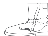
The upper shows deformations or abrasions at the seams
