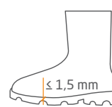
The height of cleats is less than 1.5 mm
