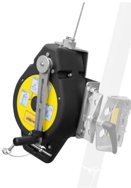
CRW 300 is a combination of a retractable type fall arrester and a rescue lifting device. The cover is made of an aluminium alloy. The arrester is fitted with retractable zinc plated steel cable. CRW 300 is fitted with rescue lifting device, and can be used independently or with selected tripods. In order to install the device on a tripod use a mounting bracket.
